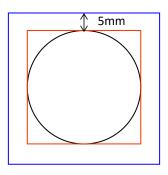
Assuming that the cutting graphic is a circle, the cutting frame graphic is a red rectangle. If the 【Blanks Distance 】 is set to 5mm, the cutting frame graphic is a blue rectangle, that is, the distance from the actual cutting frame position is 5mm.
