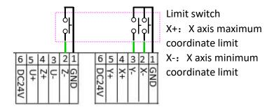
When the selected limit switch is a normally open limit switch, the voltage of the limit signal input port is 24V. After the limit switch is touched, the voltage of the limit signal input port becomes 0V, and limit-switch valid level is low-level. When the selected limit switch is a normally closed switch, the voltage of the limit signal input port is 0V. After the limit switch is touched, the voltage of the limit signal input port is 24V, and limit-switch valid level is high-level.
