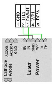
**Note:** When the laser is a radio frequency tube, there is no need to connect to the TTL port, just connect to the PWM port to control the laser switch and power; when the laser is a CO2 glass tube, you need to connect the TTL and PWM ports at the same time, which are responsible for the laser switch And power.
