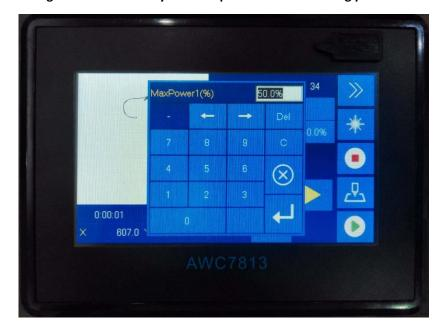
Figure 3-10-2-1 Modify the max power of the file being processed
