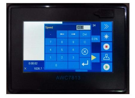
Figure 3-9-2 Modify the speed of the file being processed
