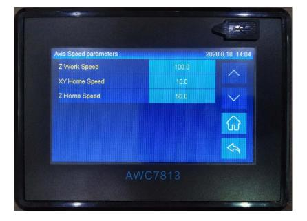
Figure 3-15-3 Axis Speed Parameters
