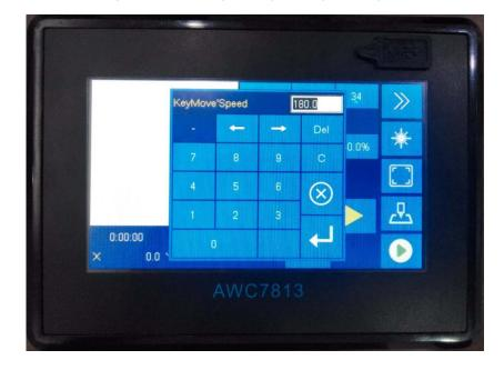
Figure 3-9-1 Quickly modify the key move speed
