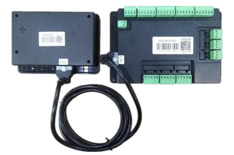
Figure 2-3-4 Connection port of panel and wiring board
