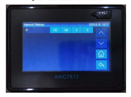
Figure 3-17-3 Set the control card IP address
