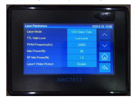
Figure 3-16-2 Laser parameters setting
