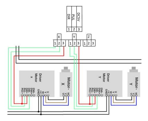
**Note:** When the Y&Z double-driver control is turned on, the Z-axis direction signal line should be connected to the Y-axis direction signal port, so that the Y&Z
