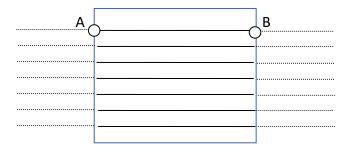
Assuming that the blue rectangle is an engraving file, the engraving track of the laser head is as shown in the figure above. To distinguish the speed, set the trajectory of the laser head idling on the outside as a dotted line, and set the trajectory of the laser head during engraving as a solid line. In order to achieve a certain engraving speed, the distance from the laser head to point A must be increased, and after reaching point B, it will be decelerated.
