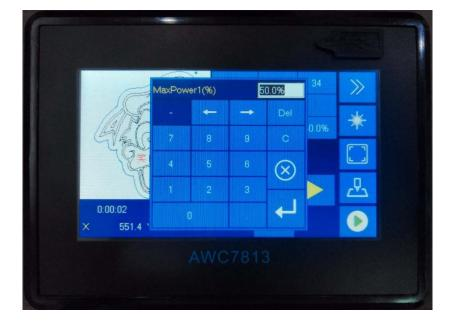
Figure 3-10-1-1 Modify the max laser power
